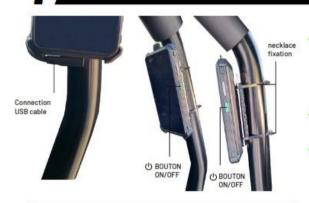
1/ Connect the USB cable to the USB port of your car and the angled part of the USB cable to the tracker IMPORTANT: The angled part of the cable must go to the left of the tracker
